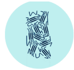
Polyethylene Irregular molecular structure (Low orientation)
